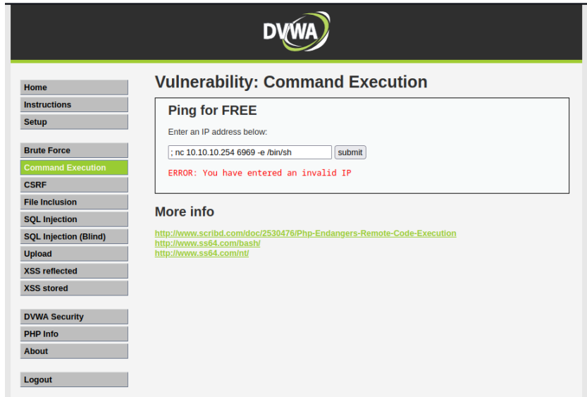
Figure 29 Command injection attack blocked
